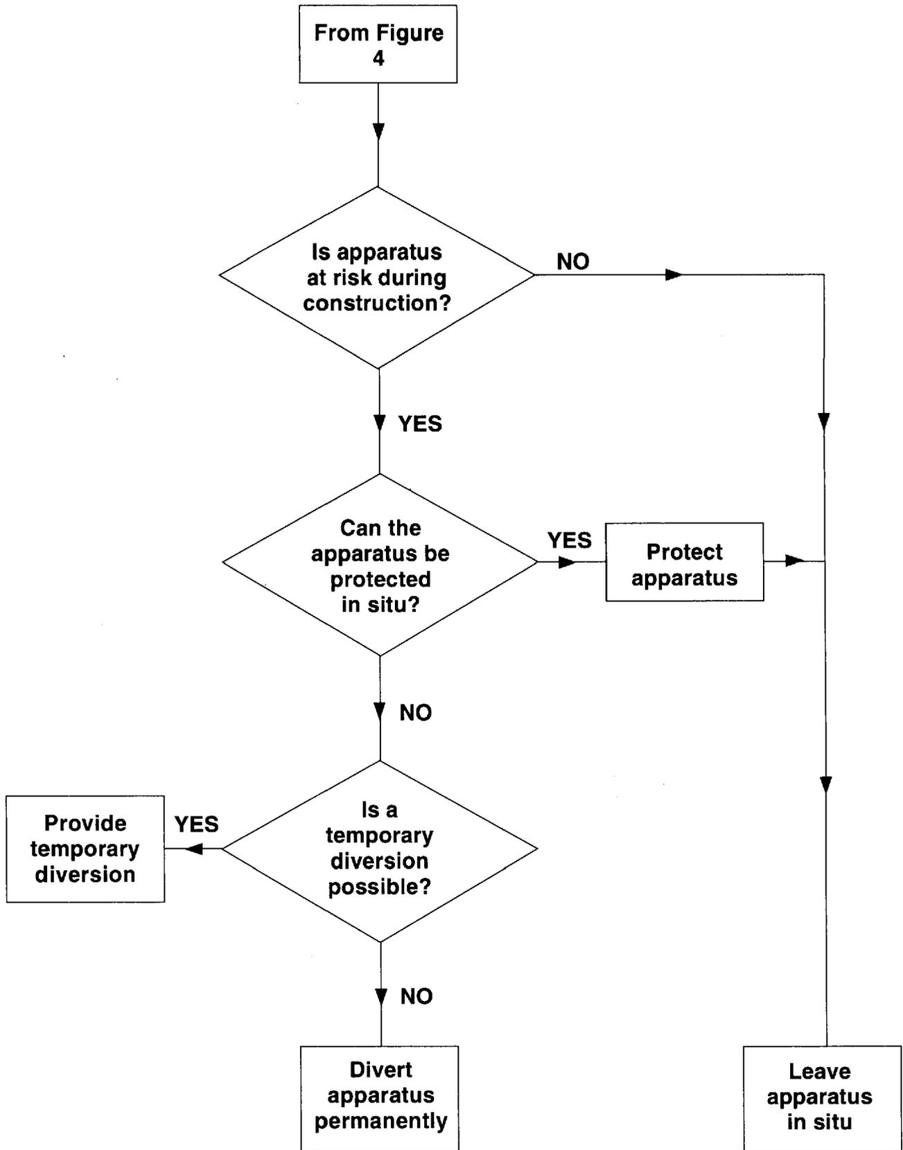
**FIGURE 3 APPARATUS AT RISK DURING CONSTRUCTION**
